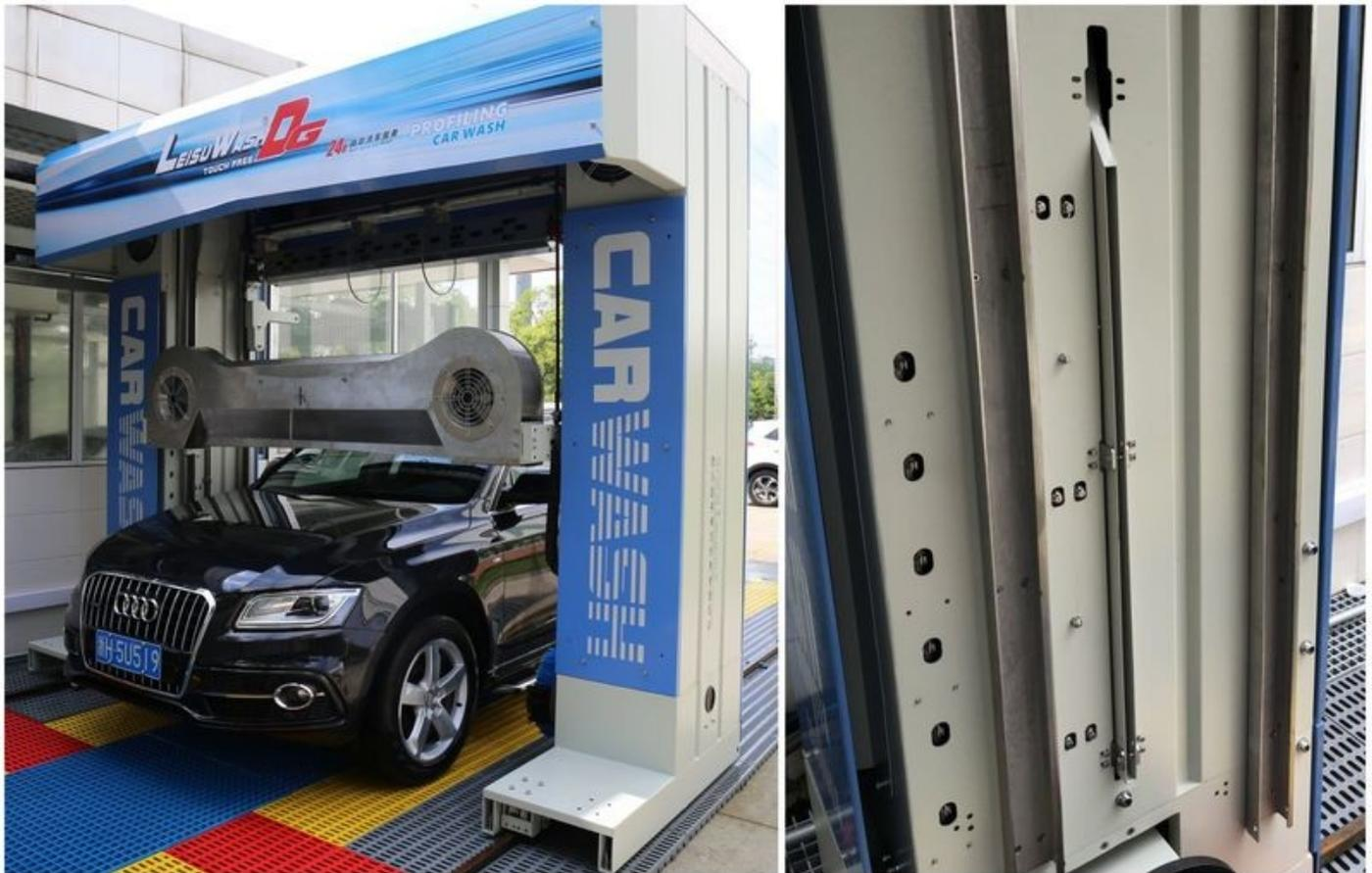
Contour-following air dryer with side air dryer
